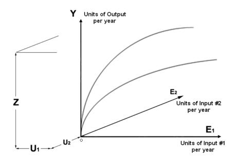
For this parametric system, an economic sector's physical output rate Y would relate to its N physical input rates E<sub>J</sub> by the following equation:
